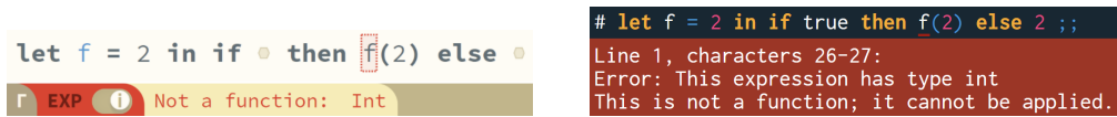
Fig. 8. Error localization of this program in Hazel and OCaml is similar, but for different reasons.
